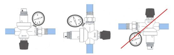
automatic filling units 111D don't get the for effects their functioning – of the gravity force; even if they can be installed in the plant in any position, we suggest not to install them up-side-down:
