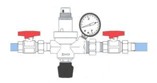
For quick installation and fast service, if requires, we recommend to install isolating valves upstream and downstream the valve.
