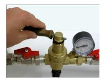
Malgorani filling units are tested before packaged: being during the proof they are pre-set at the outlet pressure of 1.5 bars; the outlet pressure can be easily modified when the valve is installed on the plant.
